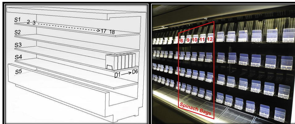
Fig. 1. Schematic of the open-refrigerated retail display case. S1–S4 represent different shelves, and D1–D6 refer to depths. S5 represents the bottom rack. The baby spinach samples were loaded in columns 8–12, and the rest of the case was filled with product simulators.
