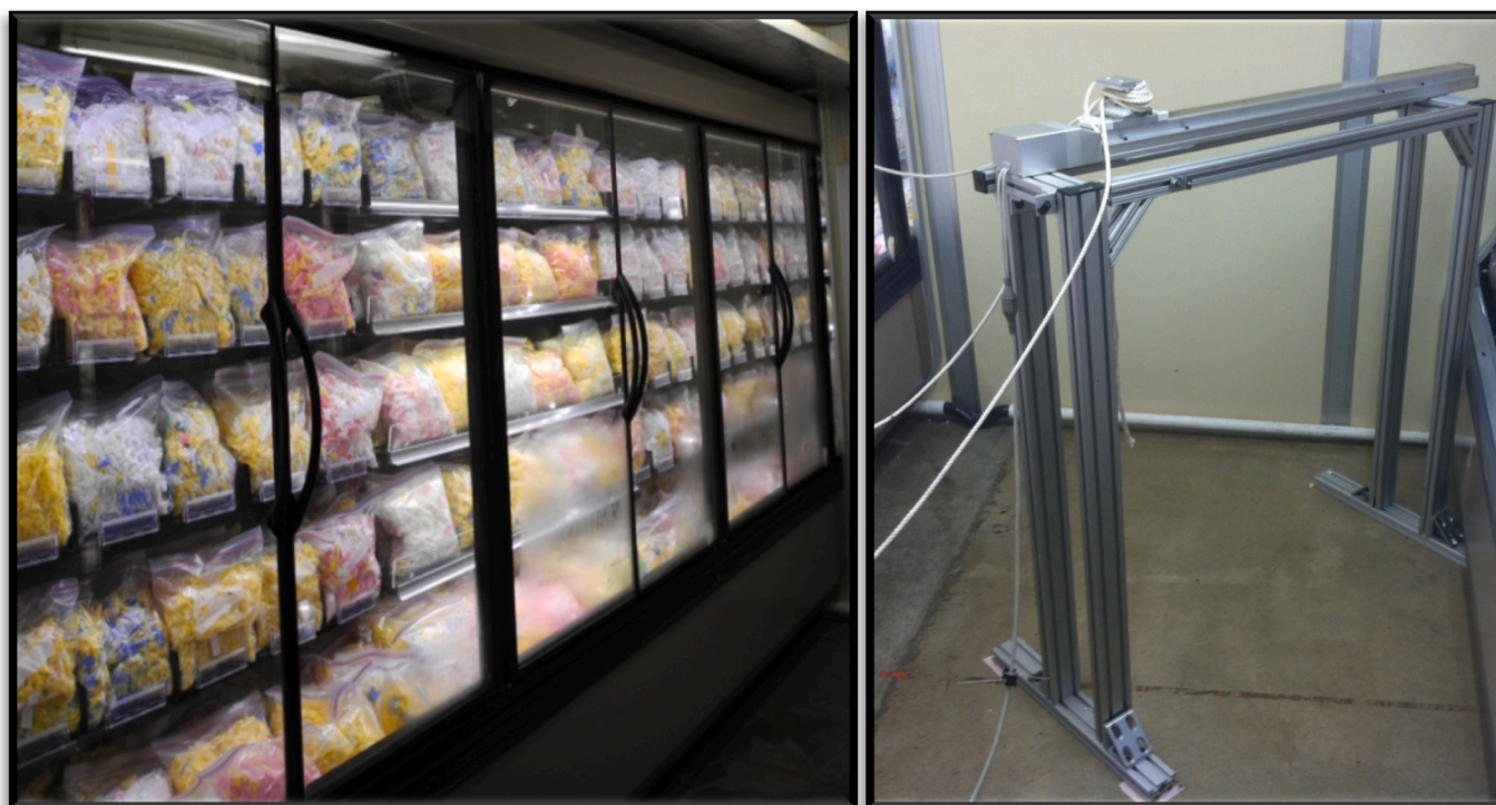
Fig. 1. Pictures of the display case with doors loaded with product simulators (left), and the automatic door opener (right). A cord is attached to the sliding arm of the door opener and three of the six display case doors.
